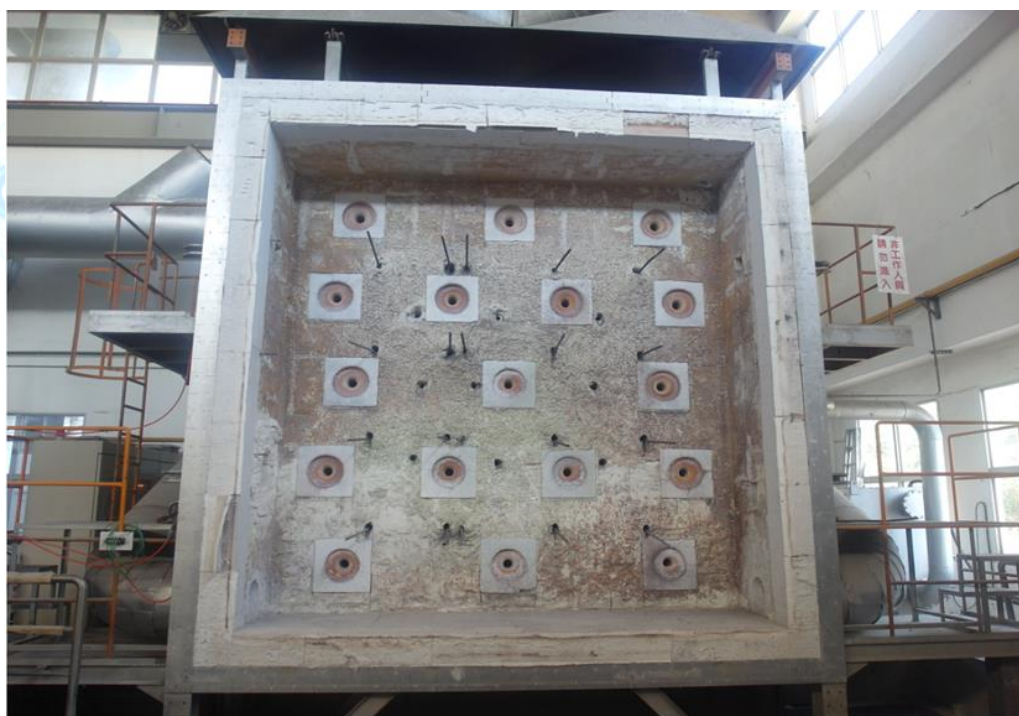
門牆耐火試驗爐(Fire-resistant test furnace on door wall)
