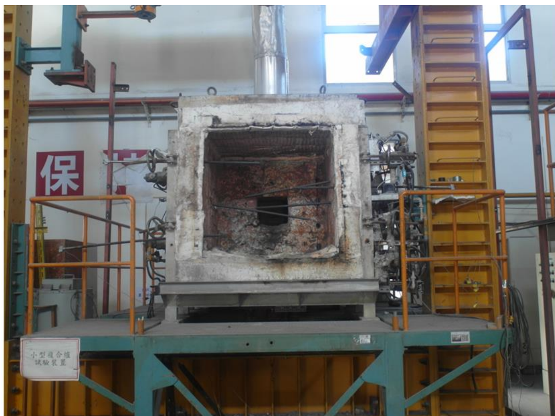
小型複合耐火爐(Small composite Fire Resistance furnace)
