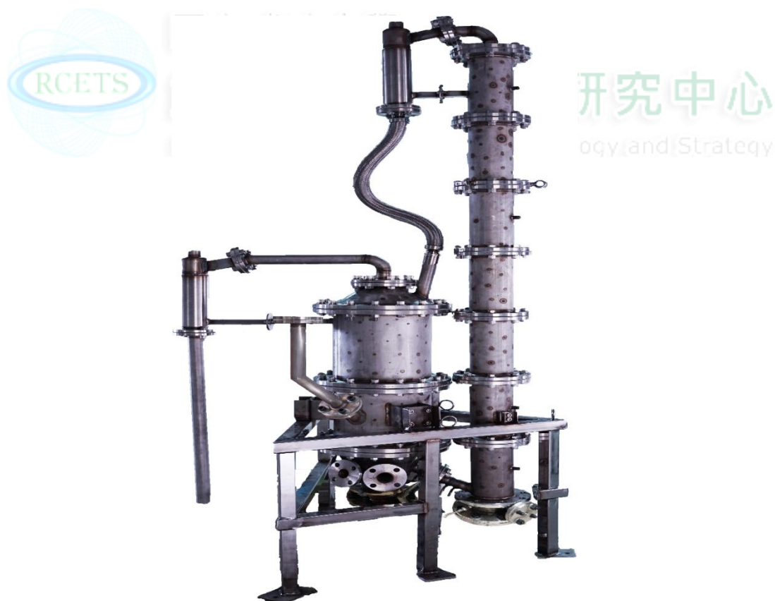
10 kWth 雙流化床氣化爐 (10 kWth Dual Fluidized Bed Gasifier)
