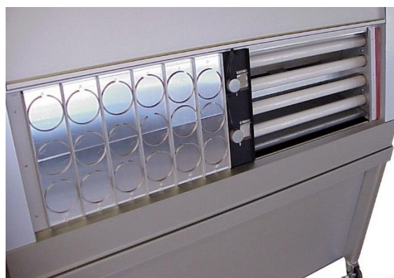
QUV 紫外光耐候試驗機(QUV Accelerated Weathering Tester)
