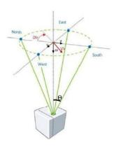
allowing to measure the wind speed at 12 different heights. The backscattered light is converted into an electronic signal and digitized. A dedicated signal processing algorithm computes wind vector components from five consecutive line of sight
